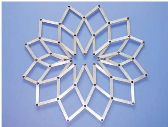
Fig. 5 Expanded and folded configurations of a mobile foldable bar structure in which the rigid plates of earlier diagrams are replaced by rigid bars.
