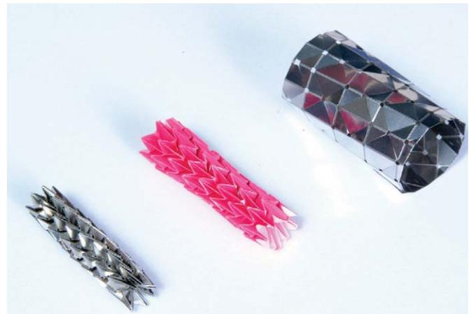
Fig. 13 Models of an origami stent graft that can be used in the treatment of oesophageal cancer. The models are made from stainless steel tubes to obtain good geometrical compatibility during expansion, though in reality much more flexible materials are used.
