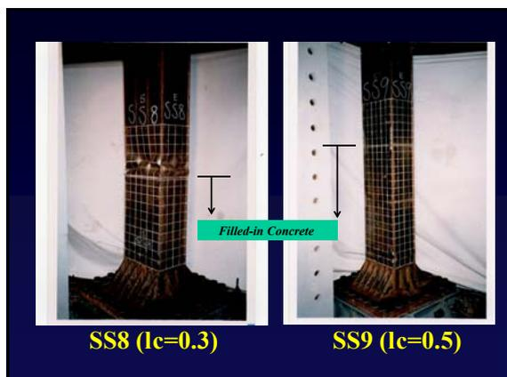
Reducing Width-thickness Ratio of Plates
