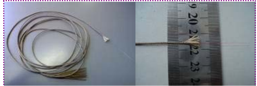
Basalt fiber packaged optical fiber sensor
